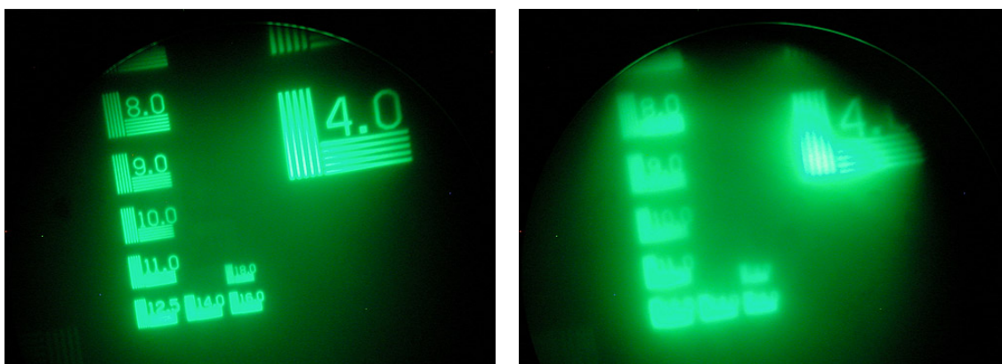
Figure 24: Fluorescence images of the projected resolution target at 10× (left) and 40× (right) demagnification.
