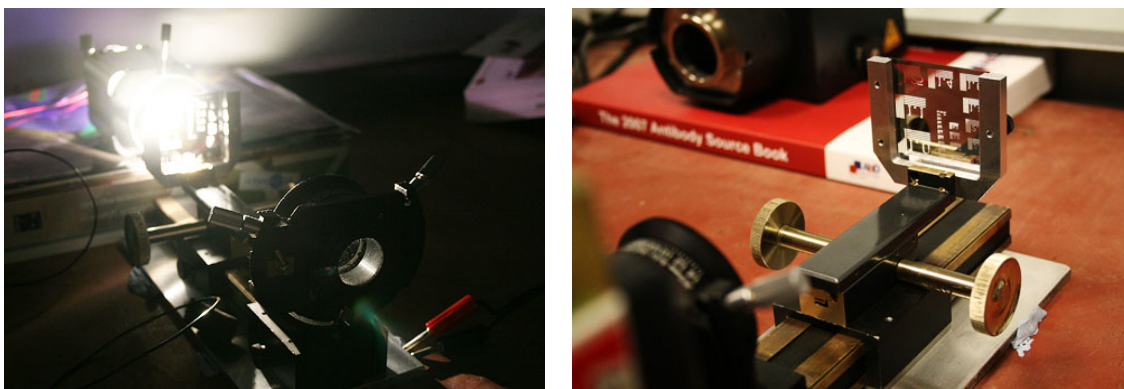
Figure 23: Projection apparatus for the imaging the NBS 1963A resolution target.
